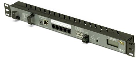
The SuperGoose II occupies a 1-U space and contains a complete set of internal sensors. A variety of remote sensors are easily added.
