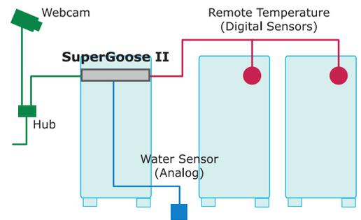
A SuperGoose II uses remote temperature sensors to monitor multiple cabinets. A water sensor checks for water leaks and a web cam provides remote images of the room.
