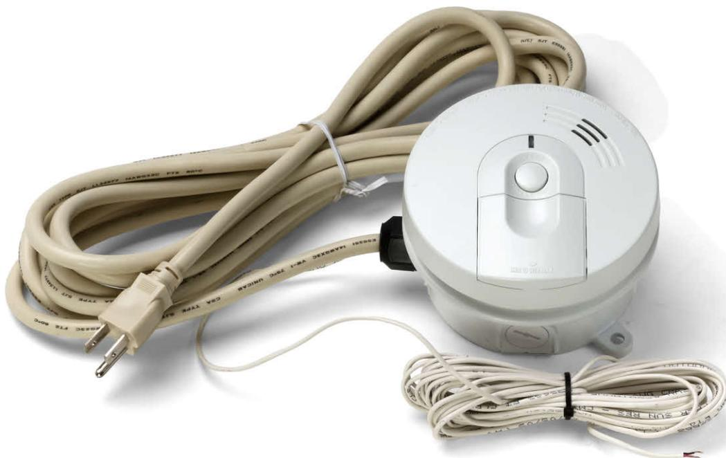
The SA-1 is powered both by a 120VAC wall plug, and by a 9V backup battery which keeps the unit alive and functioning in the event of a line-power failure. This means that as long as your WeatherGoose and its associated network & internet gateways are also kept alive via a UPS or auxiliary generator during a power failure, then you will still receive e-mails and/or SNMP trap events if smoke should be detected.
