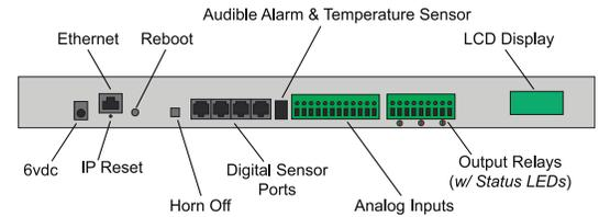
The RelayGoose II occupies a 1-U space, provides environment monitoring and contains output relays controlled either manually or triggered by alarm.
