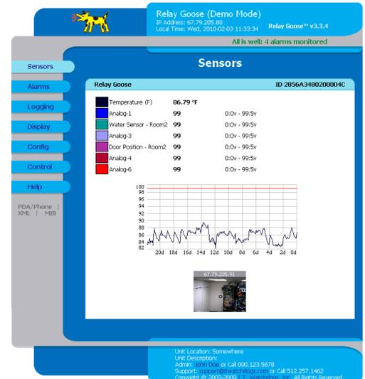
View current sensor readings and graphs on the Sensors page. The names of the analog inputs are user-defined.
