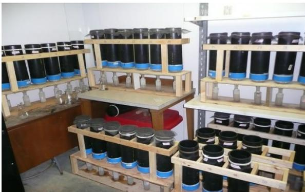
Soil columns in lab chamber
