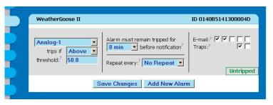
actions you wish this alarm threshold to trigger, along with a trigger delay or alarm-repeat interval if desired, and click *Save Changes*. The alarm will trip when the switch contacts open, allowing the reading to rise from "0" to "99", and clear when the switch contacts close and the reading returns to "0".
