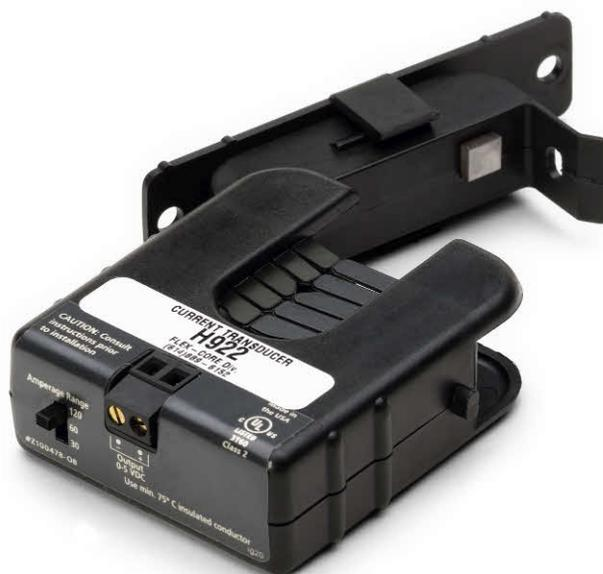
Note that for the current transformer to work properly, it is necessary that only the “hot”, current-carrying wire passes through middle of the transformer; if the CT is simply clamped around a standard 2-wire or 3-wire power cord, you won’t get any reading.
