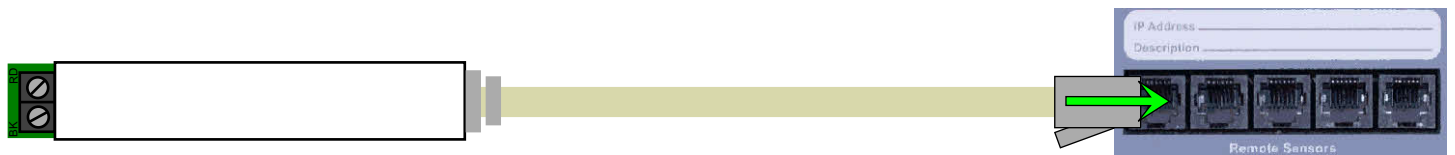
modular plug at the end of the CCAT data cable fits into one of the corresponding jacks on the WeatherGoose monitoring unit
