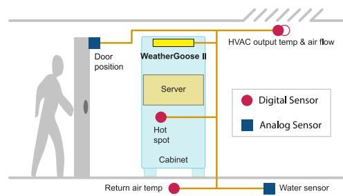
*This server room uses a WeatherGoose II to monitor the cabinet environment plus five external sensors to monitor the A/C output, cabinet hotspots, return air temperature, water leaks and door position.*
