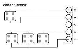
Water Sensors wired in parallel
