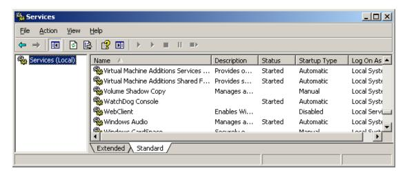
9. Check to see if any startup errors have occurred by checking the C:\Documents and Settings\All Users\Application Data\WatchDog Console\data to see if a file named errors.log has been created there. If so, open the file and diagnose the problem.
