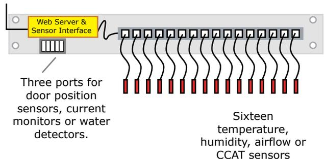
*A single MiniGoose can monitor up to 17 individual cabinets. The remote sensors should be placed in the hottest location in the cabinet.*
