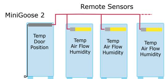
*External sensors connect using Cat 3 telephone cable and RJ-11 connectors and a splitter. The aggregate cable length should not exceed 600'.*
