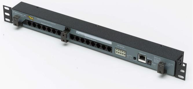
*The MiniGoose 2 is rack-mounted and contains an internal temperature sensor plus two types of remote sensor inputs. A three input I/O jacks permit door monitoring and current monitoring. Additionally, 16 receptacles provide monitoring of remote temperature, humidity, and air flow. Contains the same alert and monitoring functions as the MiniGoose 1.*
