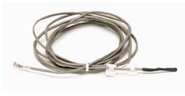
Using RJ-11 connectors and Category 3 cable the temperature sensor includes two nylon mounting clips. The sensor comes in two cable lengths, 20 and 100 feet. Total aggregate cable length limit is 600 feet.
