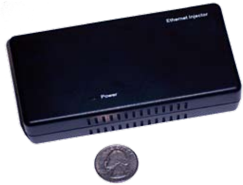
PoE Injector. Weight 200g, 117 x 60 x 35mm. Combines 120VAC with data. Output is CAT5 cable up to 300'. Power cord included.
