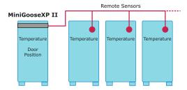
A single MiniGooseXP II wth remote **digital** sensors, can monitor up to 17 cabinets. The total aggregate cable length for **digital** sensors should not exceed 600'.
