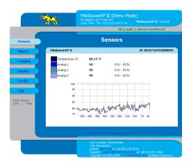
Readings from the internal temperature sensor and analog inputs are shown on the Sensors page. Page 2 of 2 Datasheet
