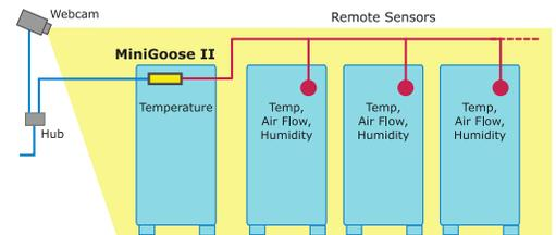
The MiniGoose II uses remote sensors to monitor multiple cabinets and interfaces with a variety of web cams.
