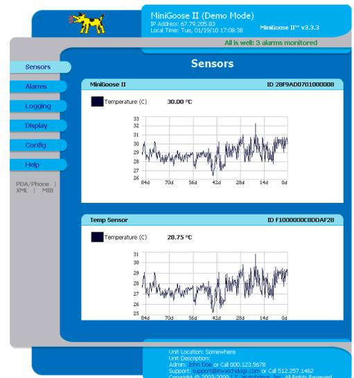
Sensor data and graphs are grouped by device, with internal sensors in the first box and remote sensors in the following boxes.
