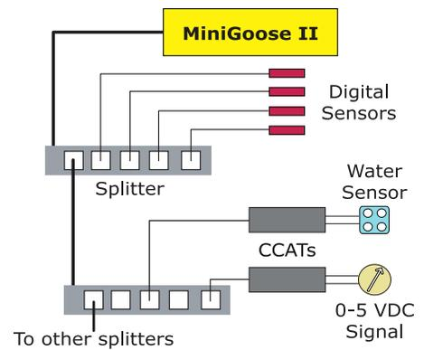
*Daisy-chain splitters and connect up to 16 digital sensors. Use a CCAT to interface an analog sensor with the MiniGoose II.*
