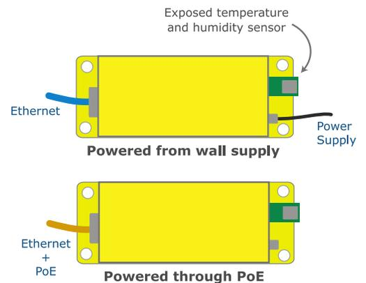
A self-contained climate monitor, the MicroGoose needs only an Ethernet connection and power. In a network with PoE, both are supplied through an Ethernet cable. Otherwise the included wall power supply is used.
