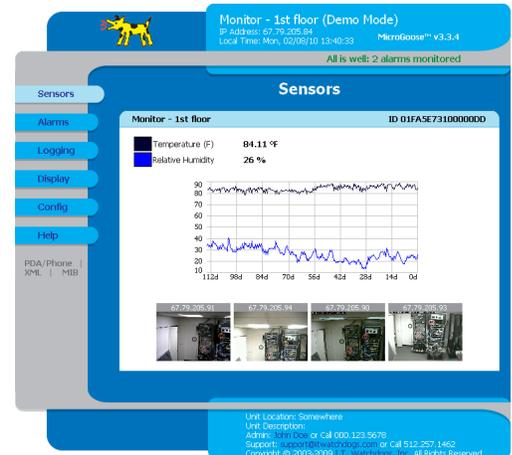
The Sensors page shows temperature, humidity and images of up to four web cams.
